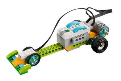
a car e.g. size of wheels and tyres, gears, weight. We learned that the bigger the tyres, the faster the car will travel a specific distance if everything else is kept the same. We built the race car following the building instructions. The car uses a pulley system to make it go. We then programmed it so that the motor would turn on and off at the appropriate times. We tested the car with big wheels and small wheels to see what differences it would create.
